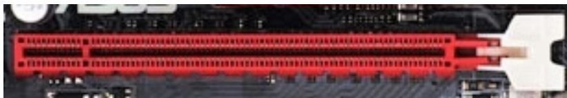
FIGURE 3.2. – Un port PCIe x16
